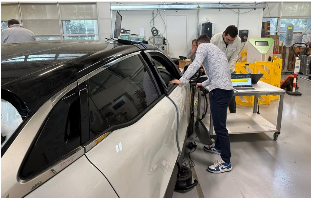
Figure 18: Successful V2G charging test WDS charger with EV onboard charger at R&D centre
