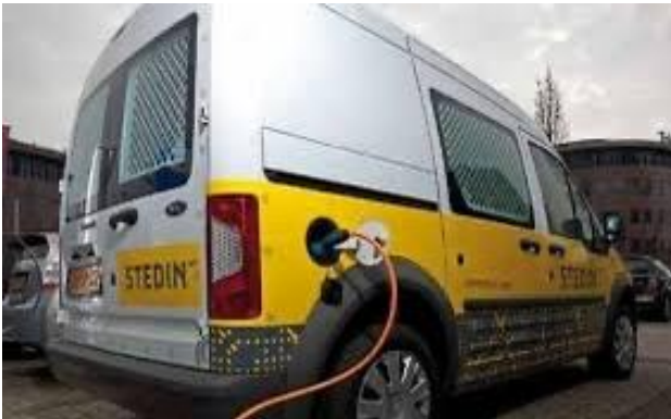
Figure 22 LCV from STEDIN in charging procedure
