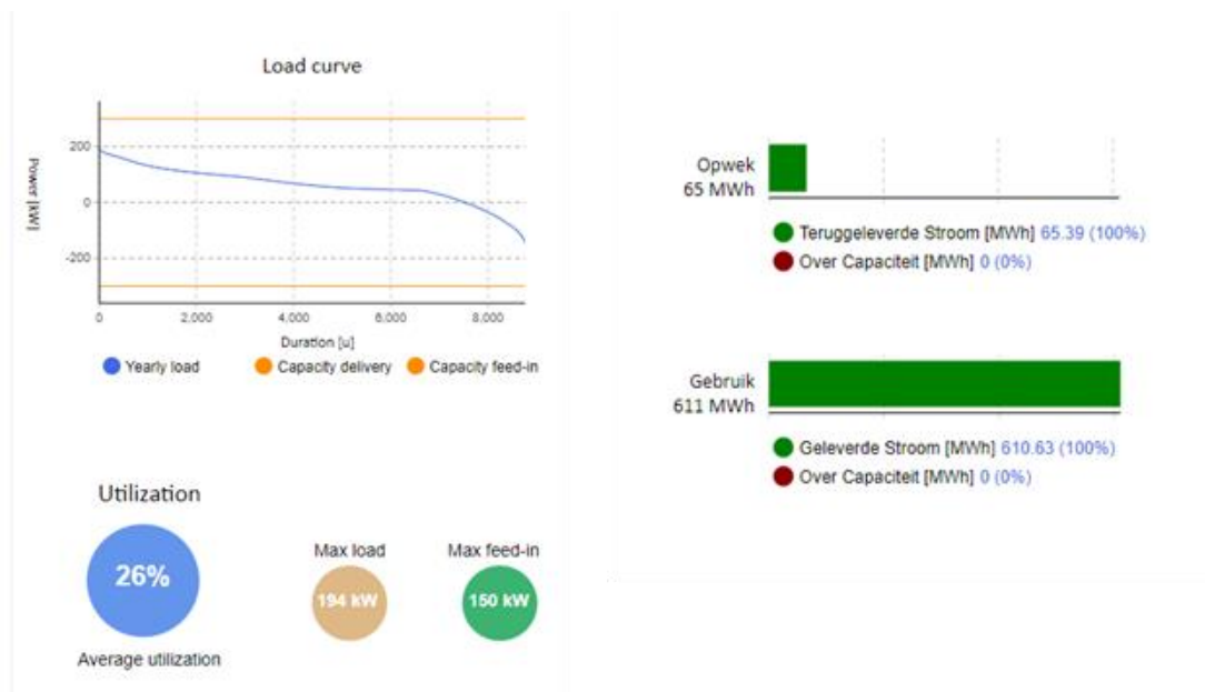
Figure 6: Examples of figures for the yearly simulation function of the tool. The left graph shows a load duration curve for a specific object. The right graph shows the annual consumption/generation volumes of a specific object.
